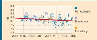
UK pH data 2008 - 2015 for time series at L4 (off Plymouth), Stonehaven (near Aberdeen) and for SmartBuoys in the North Sea and Irish Sea, the red line illustrates the trend. Modified from Ostle *et al.*, 2016, Carbon dioxide and ocean acidification observations in UK waters: Synthesis report with a focus on 2010 - 2015. doi:10.13140/RG.2.1.4819.4164
