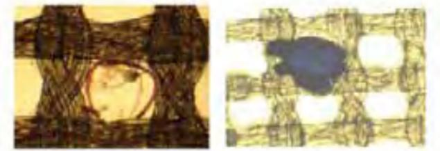
Figure 17. Examples of microplastic debris found in CPR samples. Nylon monofilament (left) and Polyethylene terephthalate fragments (right). Scale bar 270  $\mu$ m.
