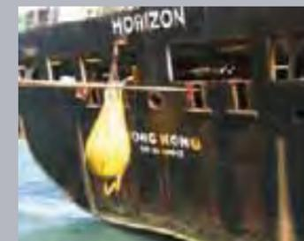
Left: Four tonnes water bag, load test on the tow point of MV *HORIZON* at Durban to give 2 tonnes safe working load. Right: Marco Worship and Hans Verheye, DEA, Cape Town, load CPRs aboard.
