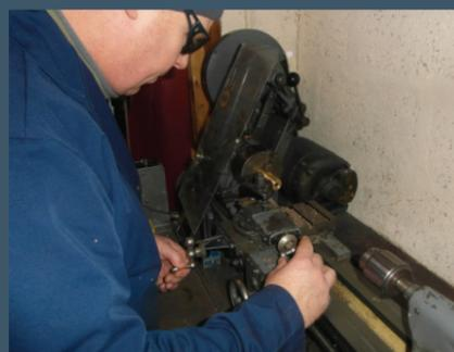
**Julian Morley**, who joined us in 2012 with a previous career as a small boats and ships engineering technician, is seen here using the lathe to produce shaft stops that are capable of being fitted with the prop protector blade. This is a device that helps keep the success rate of the CPR high in sea areas with increased detritus.
