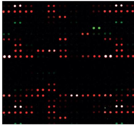
Figure 27: Example of microarray detection system on a SAHFOS sample. Coloured circles represent DNA probes that have positively detected a species. With 140 probes multiple species can be detected on the array- red and green colours indicate intensity of detection. There are many duplicate probes of any one taxa embedded within this microarray test to prevent false positive detection, providing a robust assay system.
