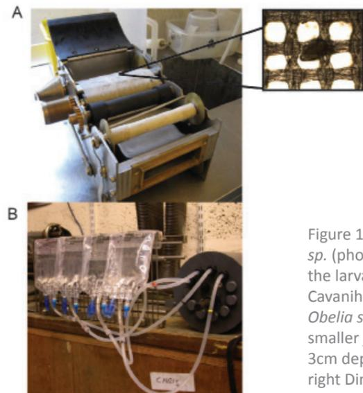
Figure 14: Panel A shows a CPR recorder with silk in it and inset showing a close-up of the silk mesh with 270µm holes. Panel B shows water sampler (WaMS) device taken apart - a pump that collects a small volume of water into plastic, medical bags.
