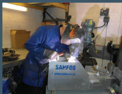
**Chris Harris**, who is an expert boiler maker by trade, is carrying out stainless steel welding repairs to a CPR that was damaged whilst being recovered in rough weather.
