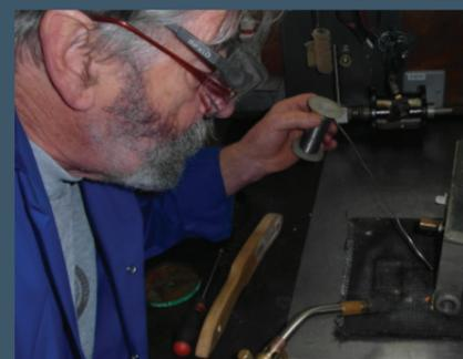
**Roger Barnard**, our long-standing CPR technician, can be seen here repairing the formalin tank on an ageing CPR. This is a particularly skilful task that requires absolute cleanliness of the components and the correct application of heat. Too much heat and the tank would fall apart.
