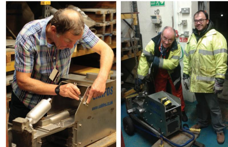
Figure 2. Testing and deployment of new instrumentation on the CPR. Anthony Walne fitting instruments for temperature, salinity, pitch & roll (far left). Peter Pritchard and Márcio da Silva Tamanaha (Univali, Brazil) looking happy after a successful late night recovery of the CPR from the PR route with all instrumentation still attached (left).
